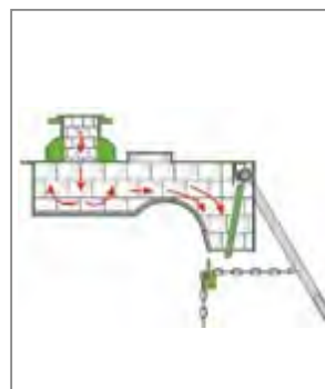
Shallow stilling feed chute
